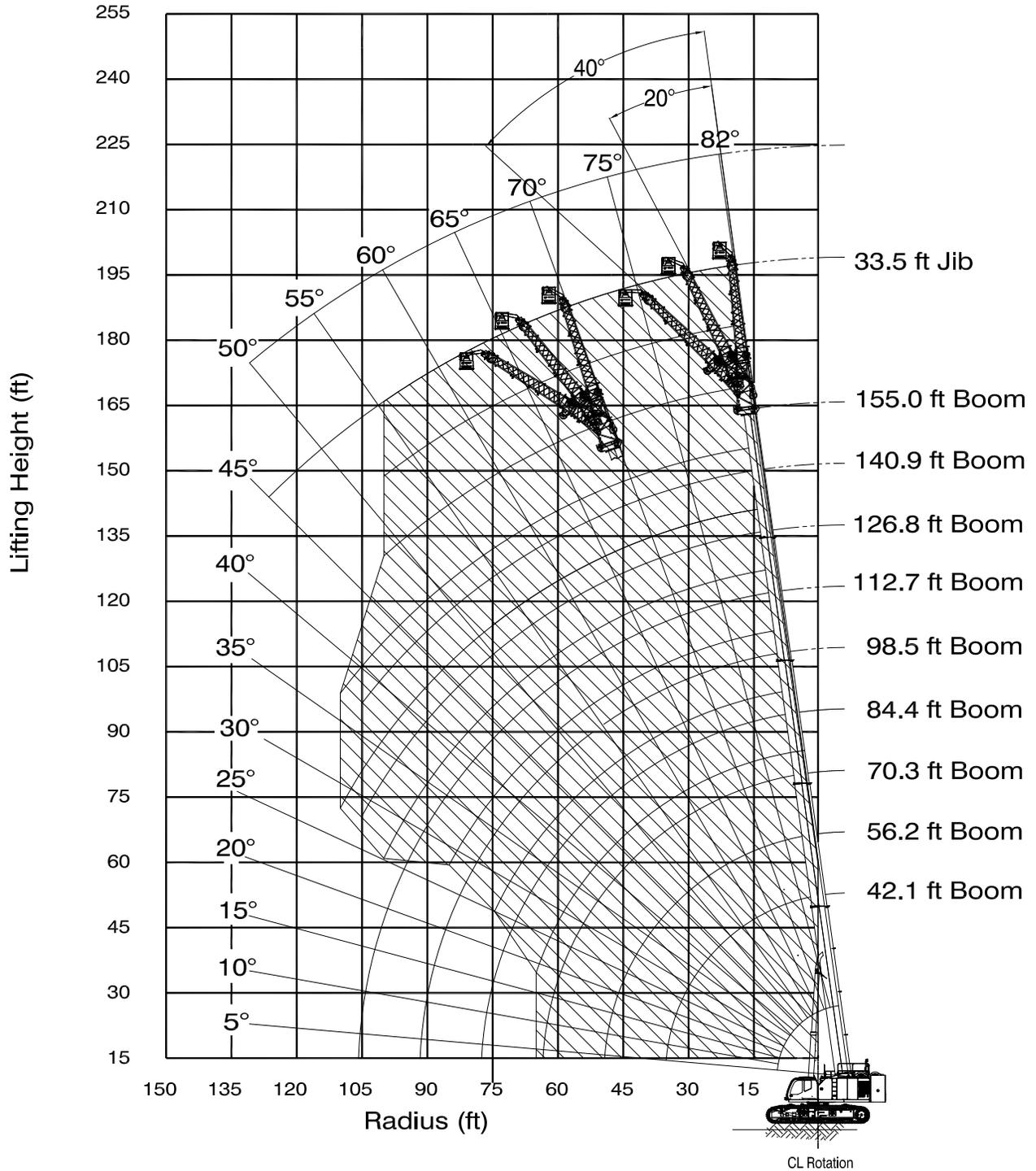
Load chart data is for reference, load charts supplied in the crane cab shall be used for lift planning.
