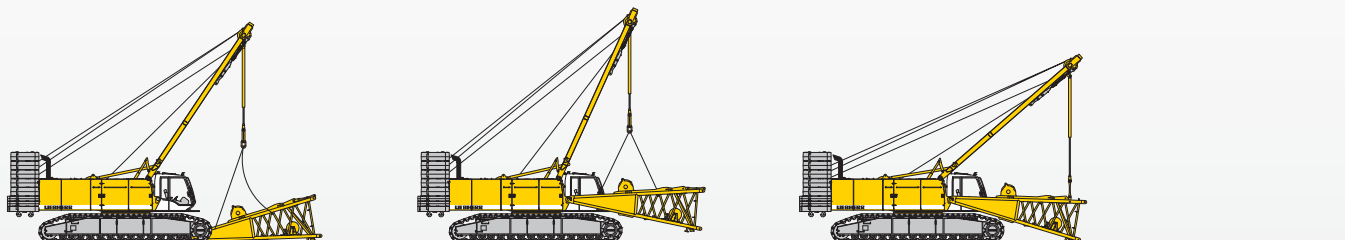
Unloading and assembly of boom foot
