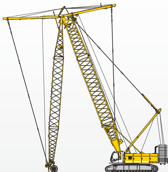
Erecting of main boom and luffing jib
