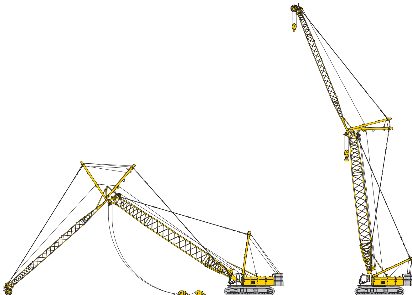
Erecting of main boom and luffing jib
